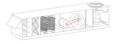
Rooftop Units (RTU) are air handlers designed for outdoor use, typically located on roofs. They are also known as packaged units (PU). The main difference is that they are usually more compact and because they are typically installed on the roof they need to be more robust and weather proof. While AHU's are often connected to a central plant such as chillers and boilers, RTU's are self contained and have everything all in one unit.
