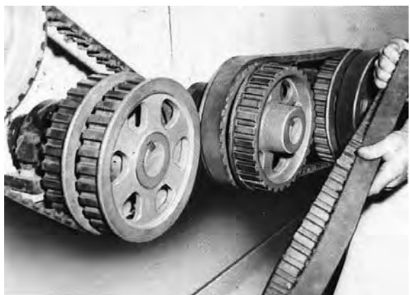
No spreader or pull-off tools are needed to replace belts.
