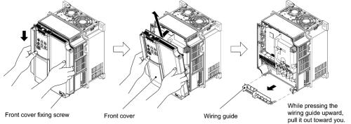
Figure 2.2: Removing the Front Cover and the Wiring Guide (e.g EQ7-4020-C)
