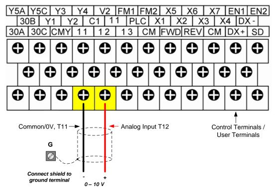
Analog Reference: Potentiometer / Speed Pot (Setting F01 = 1):
