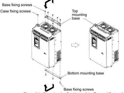
Figure 2.1: Changing the Positions of the Top and Bottom Mounting Bases
