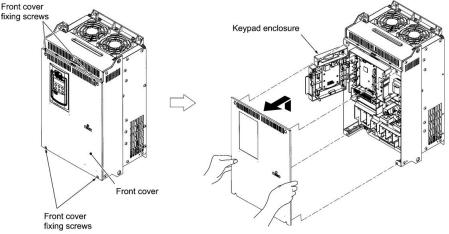
Tightening torque: 15.9 lb-in (1.8 N•m) (M4) 31.0 lb-in (3.5 N•m) (M5)
