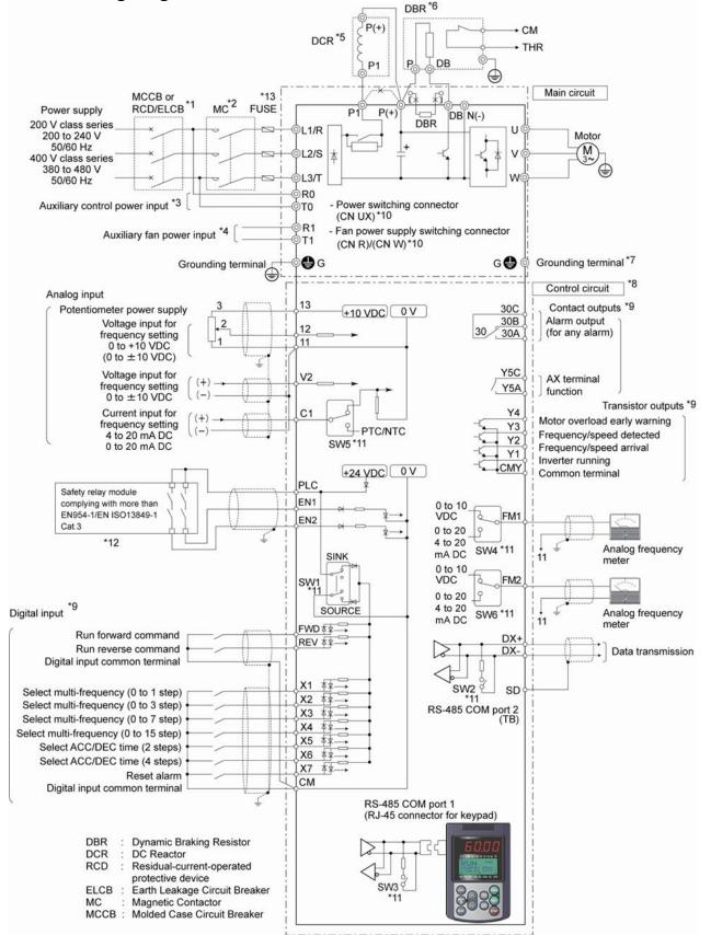
\*1 Install a recommended molded case circuit breaker (MCCB) or residual-current-operated protective device
