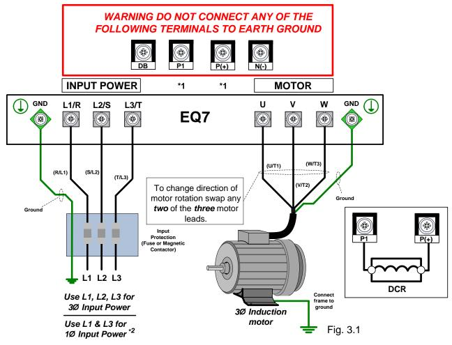
\*1. Refer to page 12 & 13 for connecting a DC reactor from the terminals P1 and P(+).
